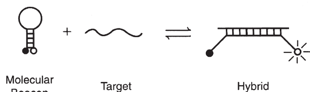
Figure 1. Operation of molecular beacons. On their own, these molecules are nonfluorescent, because the stem hybrid keeps the fluorophore close to the quencher. When the probe sequence in the loop hybridizes to its target, forming a rigid double helix, a conformational reorganization occurs that separates the quencher from the fluorophore, restoring fluorescence.
